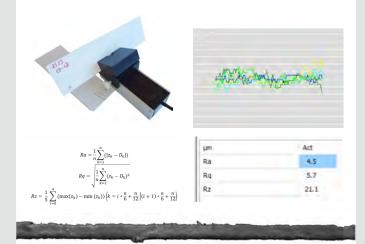
Measure the sharpness of cutting edges to reduce the dust in the press room.
