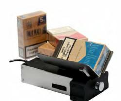
The easy way to align a finished box properly for folding angle measurement
